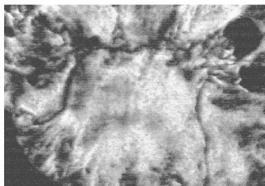
Figure 4. POM optical texture of a mixture of 70/30 (w/w) 1 /1.0M HCl at ambient temperature.
